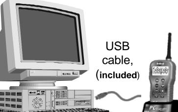
The remote relays commands and programming from the computer to the controller.
