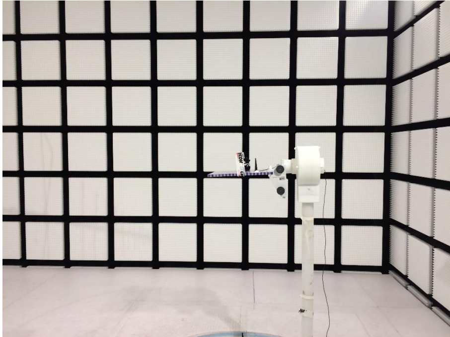
Photo 1 (RSE set-up / fully-anechoic chamber):
