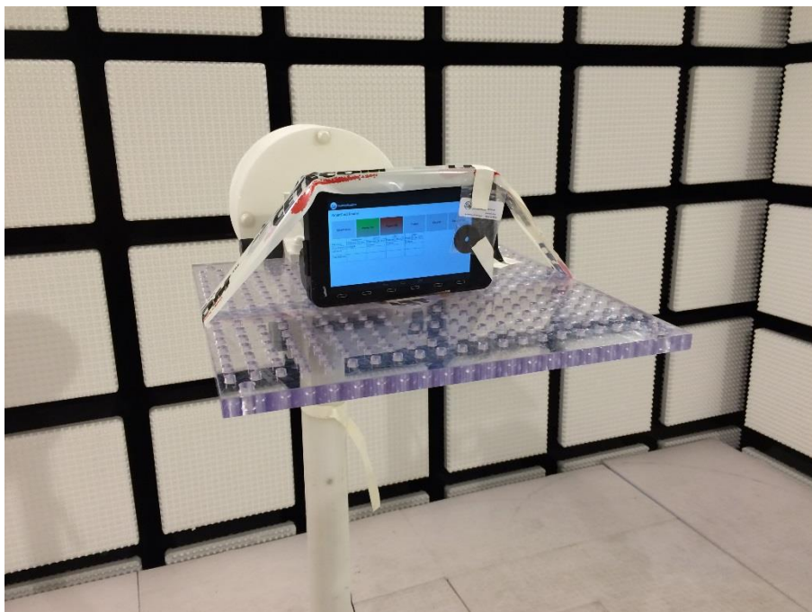
Photo 4 (RSE set-up / fully-anechoic chamber):
