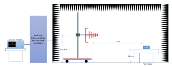
Radiated Setup 1GHz - 18GHz
