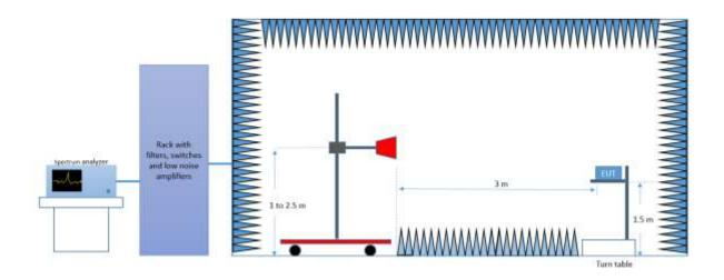
Radiated Setup 18 GHz - 25 GHz
