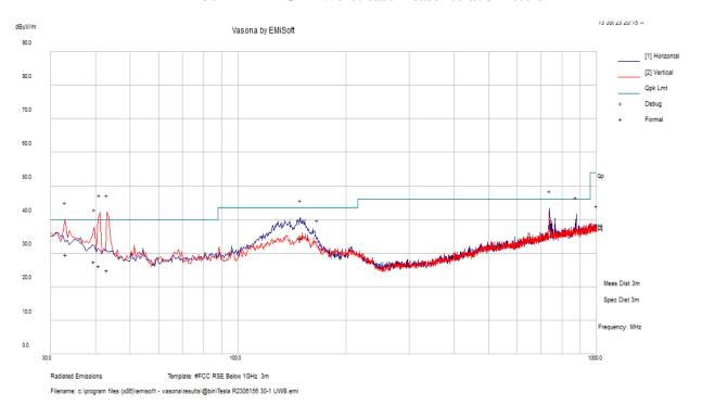
**Turntable** Corrected Antenna S.A. Corr. Antenna Freq. Limit Margin Reading **Factor** Amp. Height **Polarity Azimuth** Comment (MHz)  $(dB\mu V/m)$ (dB)  $(dB\mu V)$ (H/V)(dB/m) $(dB\mu V/m)$ (cm) (degrees) 43.0883 34.52 -9.63 24.89 240 V 352 40 -15.11 QP 40.9348 34.54 -8.41 26.13 281 V 146 40 -13.87 OP 33.0178 32.54 -2.9429.6 282 V 45 40 -10.4QP 39.5805 35.06 -7.58 27.48 297 V 241 40 -12.52 QP 739.391 33.3 1.73 35.03 215 Η 45 46 -10.97 QP 149.238 42.6 -8.19 34.41 177 Η 288 43.5 -9.09 QP
