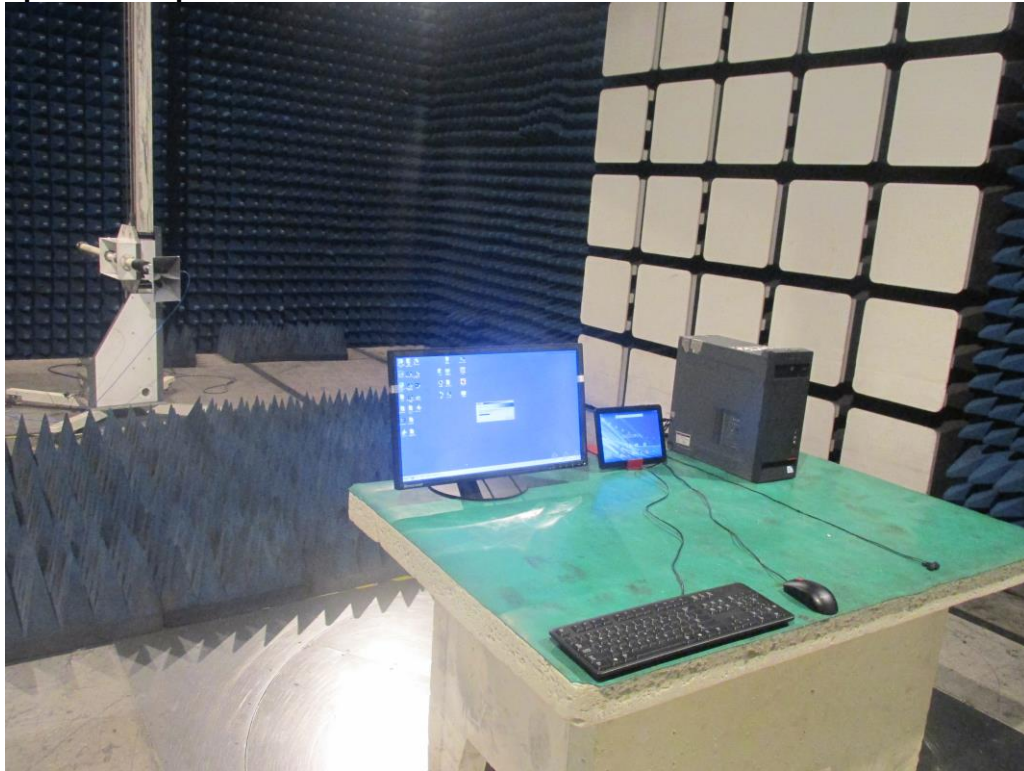
Photograph 3: Set-up for Radiated Emission of above 1GHz
