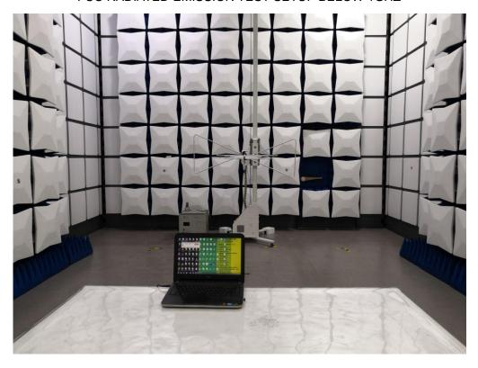
FCC RADIATED EMISSION TEST SETUP ABOVE 1GHZ
