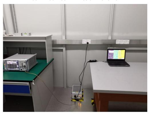
FCC RADIATED EMISSION TEST SETUP BELOW 1GHZ
