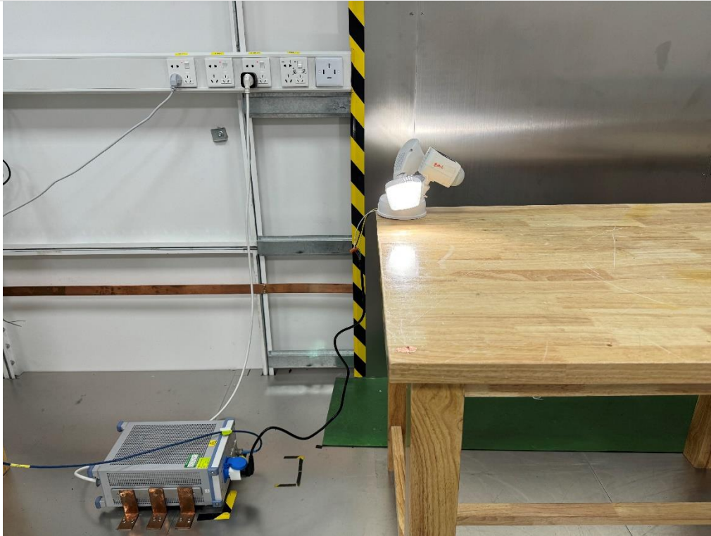
AC Power Line Conducted Emission
