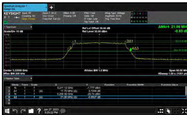
Figure 217 - 802.11n HT20 Minimum 99% OBW
