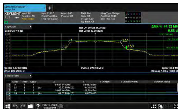
Figure 270 - 802.11ac HT40 Maximum 99% OBW
