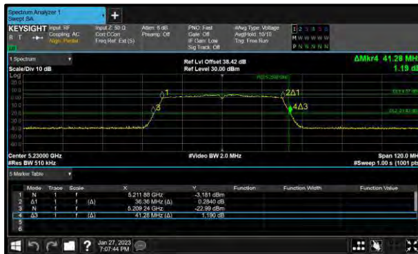
Figure 247 - 802.11n HT40 Minimum 99% OBW
