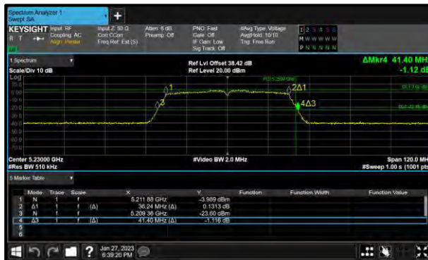
Figure 219 - 802.11n HT40 Minimum 99% OBW
