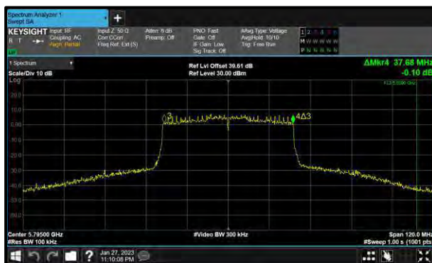
Figure 241 - 802.11ax HE40 SU Minimum 6 dB EBW
