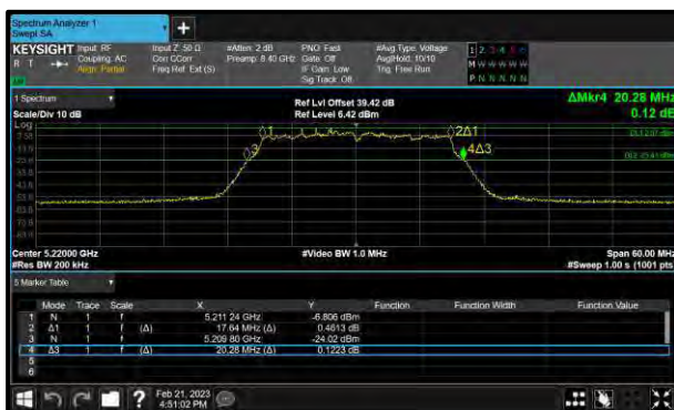
Figure 267 - 802.11ac HT20 Minimum 99% OBW
