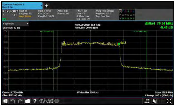
Figure 243 - 802.11ax HE80 SU Minimum 6 dB EBW
