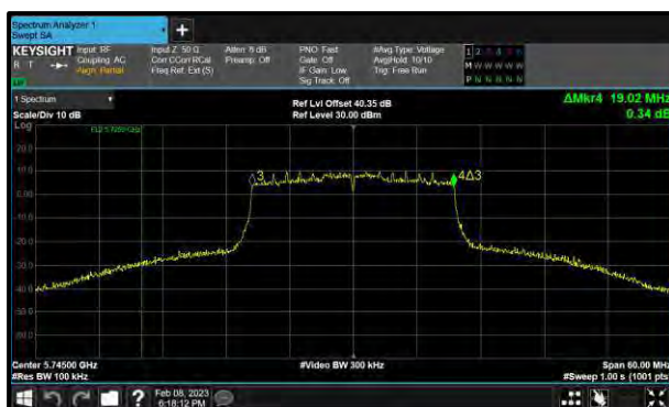
Figure 181 - 802.11ax HE20 SU Minimum 6 dB EBW
