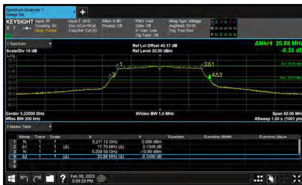
Figure 189 - 802.11n HT20 Minimum 99% OBW
