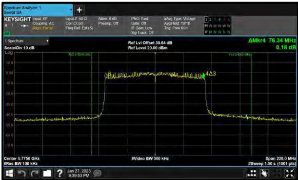
Figure 215 - 802.11ax HE80 SU Minimum 6 dB EBW
