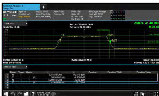
Figure 191 - 802.11n HT40 Minimum 99% OBW
