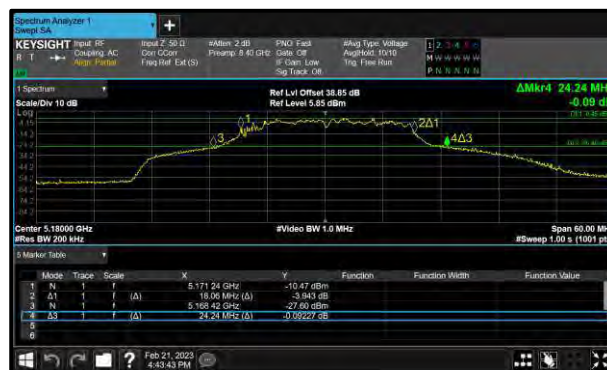
Figure 268 - 802.11ac HT20 Maximum 99% OBW
