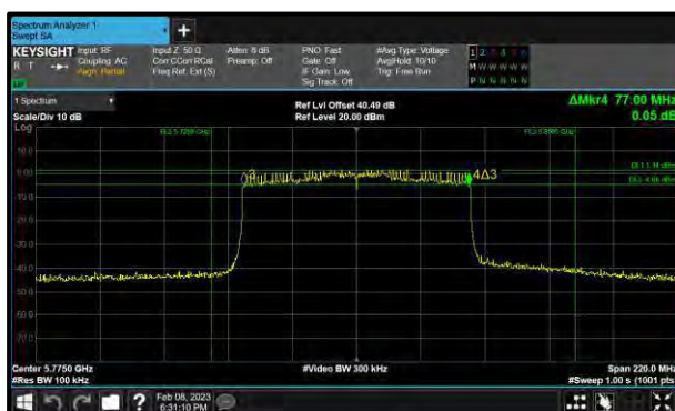
Figure 185 - 802.11ax HE80 SU Minimum 6 dB EBW
