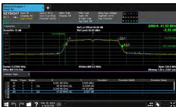
Figure 269 - 802.11ac HT40 Minimum 99% OBW
