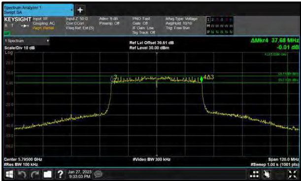
Figure 213 - 802.11ax HE40 SU Minimum 6 dB EBW
