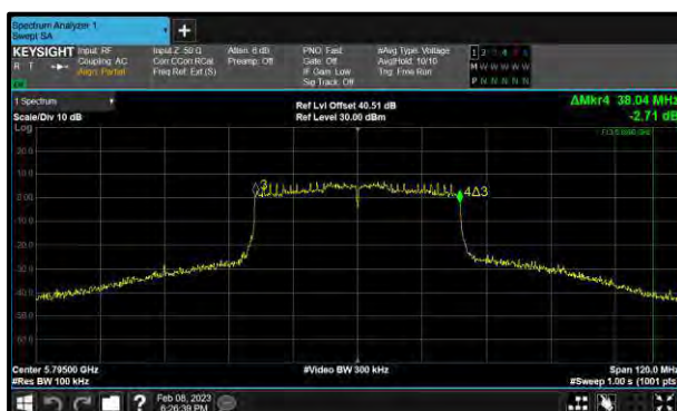
Figure 183 - 802.11ax HE40 SU Minimum 6 dB EBW
