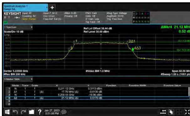
Figure 245 - 802.11n HT20 Minimum 99% OBW
