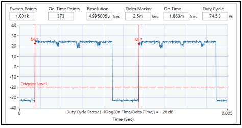
Note: The duty cycle value is 74.53%, add 10log(1/duty cycle) to the measured power level to compute the average power during continuous transmission.
