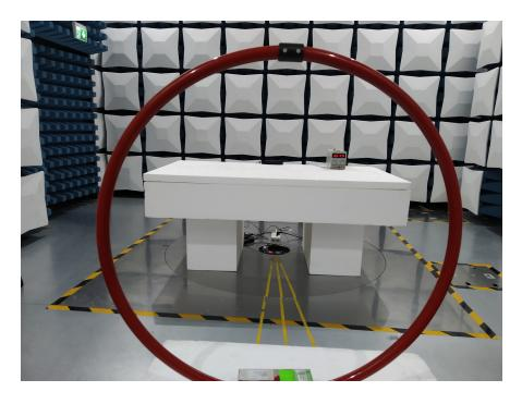
Radiated Emissions (9kHz - 30MHz)
