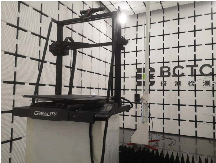
Spurious Emission Test Setup (above 1GHz)
