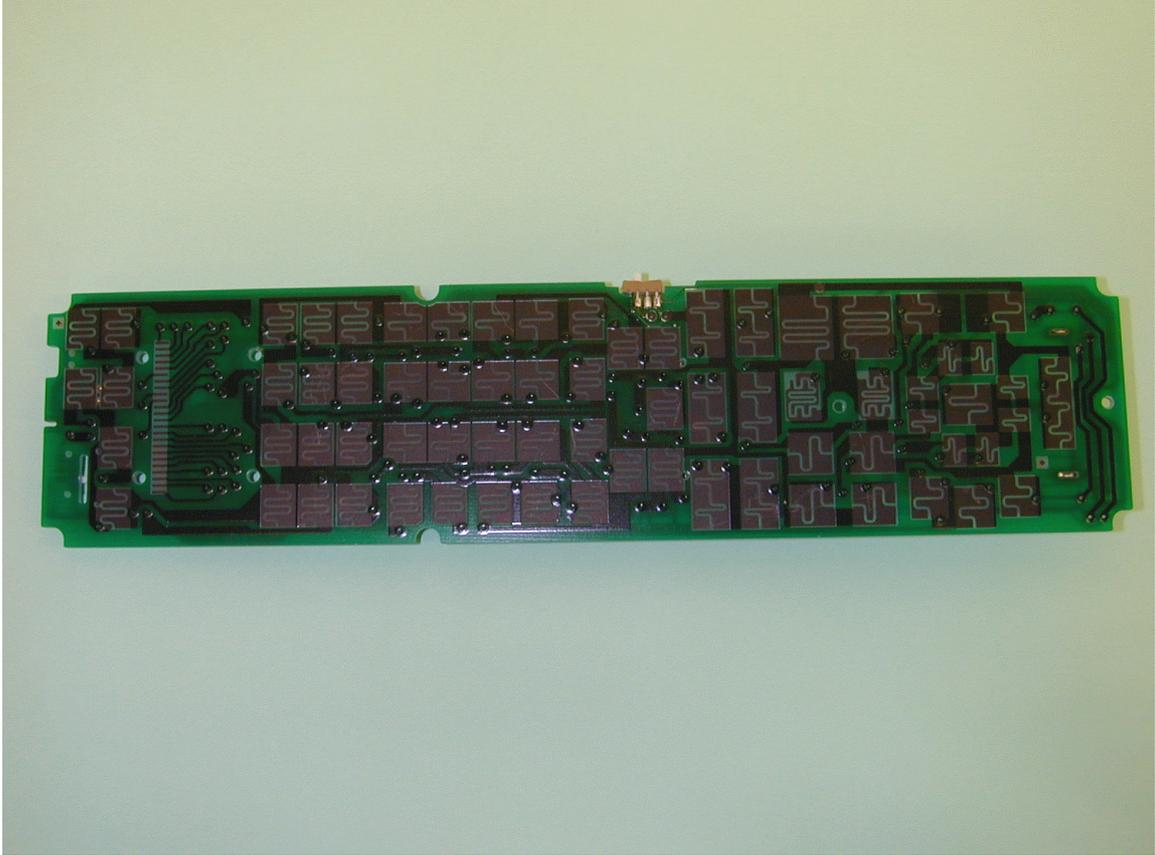
Fig. D-3 Bottom View of Main Unit RM-SRX9010J
