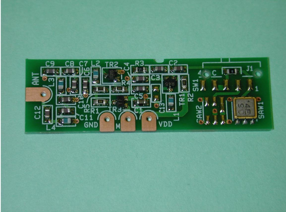
Fig. D-5 Bottom View of RF Unit RM-SRX9010J
