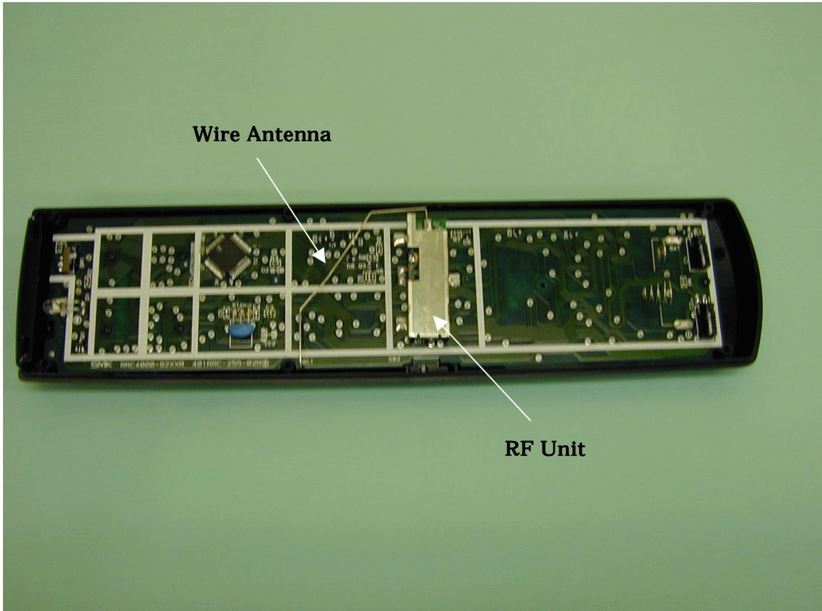
Fig. D-4 Top View of RF Unit of RM-SRX9010J
