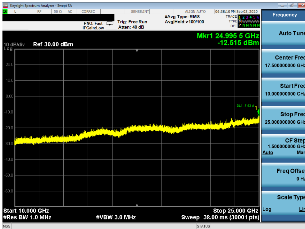
Plot 7-30. Conducted Spurious Plot (802.11b – Ch. 11)
