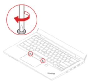
13. Take the new TrackPoint buttons out of the new keyboard package. Install the TrackPoint buttons as shown.
