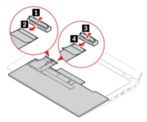
9. Attach the connectors and then turn over the keyboard.
