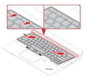
11. Slide the keyboard in the direction as shown. Ensure that the latches are secured under the keyboard frame.
