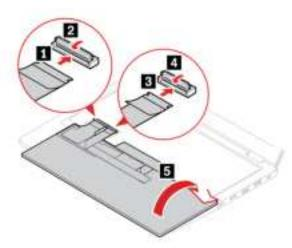
10. Insert the keyboard into the keyboard bezel as shown. Ensure that the top edge of the keyboard (the edge that is close to the display) is under the keyboard bezel.
