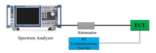
Note: The Insertion loss of the RF cable, Attenuators was offset into the Spectrum Analyzer.
