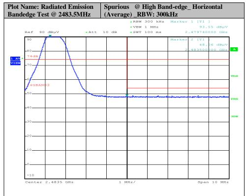
Max. Bandedge Emission by Marker-Delta Method: 94.64- (93.55-48.06)=49.15dBuV/m under the limit of 54dBuV/m.
