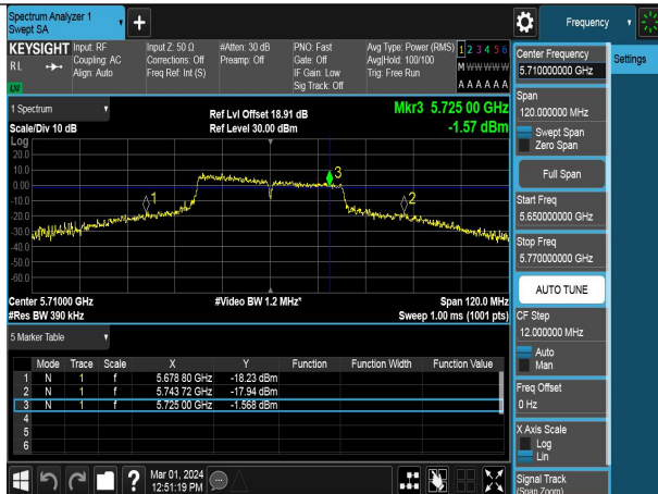
Mode:802.11ac VHT40 Frequency:5710MHz Ant:Chain0 scope:NII2C
