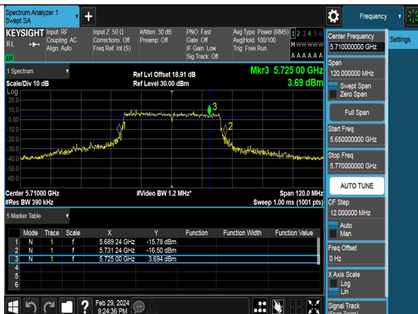
Mode:802.11ax HE40 Frequency:5710MHz Ant:Chain0 scope:NII2C
