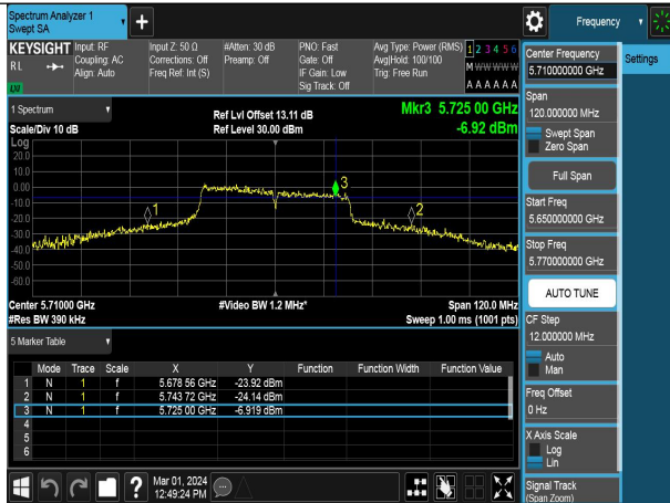
Mode:802.11n HT40 Frequency:5710MHz Ant:Chain0 scope:NII2C
