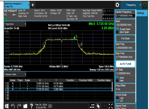
Mode:802.11ac VHT40 Frequency:5710MHz Ant:Chain1 scope:NII2C
