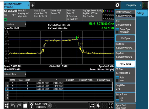
Mode:802.11ac VHT80 Frequency:5690MHz Ant:Chain1 scope:NII2C
