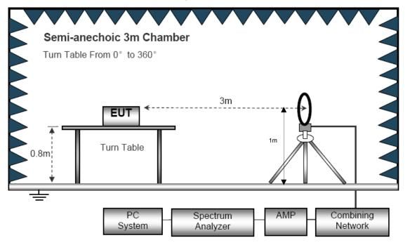
(B) Radiated Emission Test-Up Frequency 30MHz~1GHz
