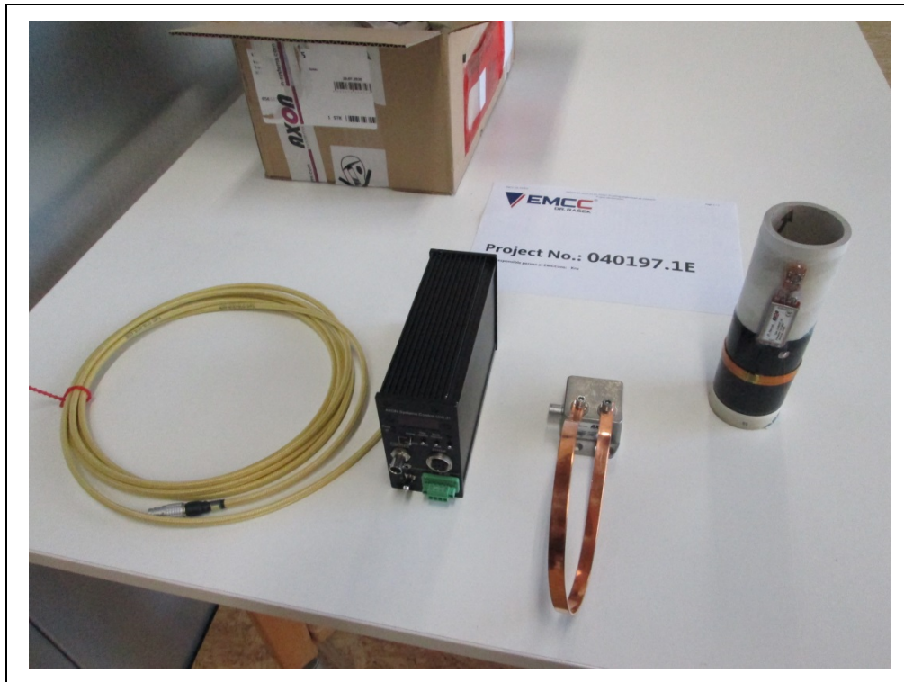
Photograph A3-13: Equipment for frequency stability tests
