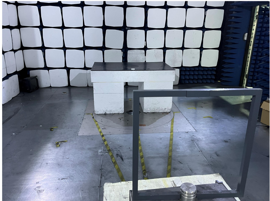
Radiation Emission Test Setup (Below 30MHz)
