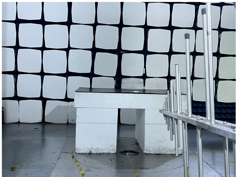
Radiation Emission Test Setup (30MHz to 1GHz)
