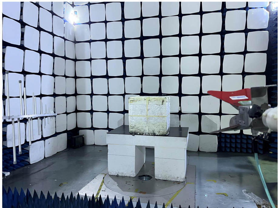
Radiation Emission Test Setup (1GHz to 18GHz)
