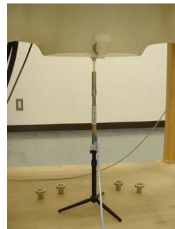
5100-5800MHz System performance check setup
