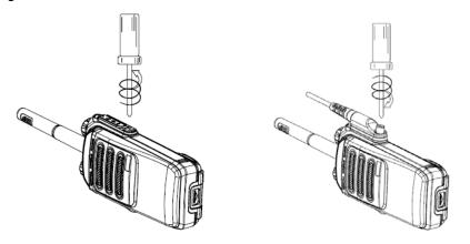
**Step 3** Tighten the screw on the connector.
