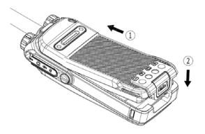
To remove the battery, turn off the radio first. Then slide the battery latch upwards (as ② shows) to
