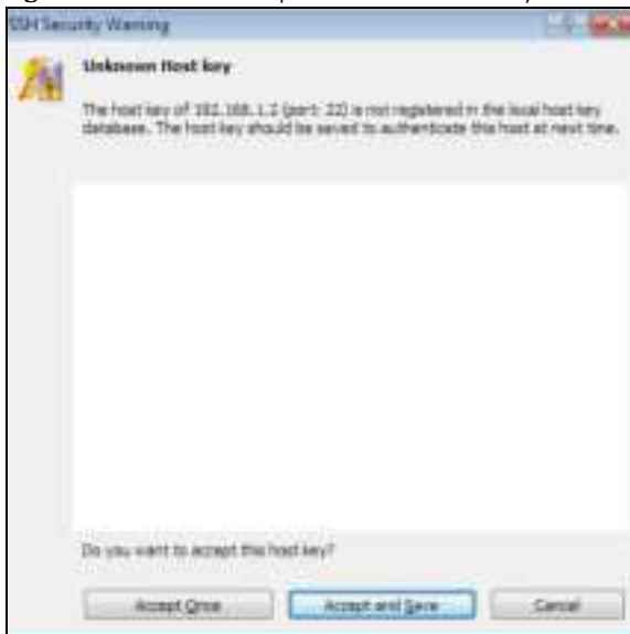
Figure 133 SSH Example 1: Store Host Key
