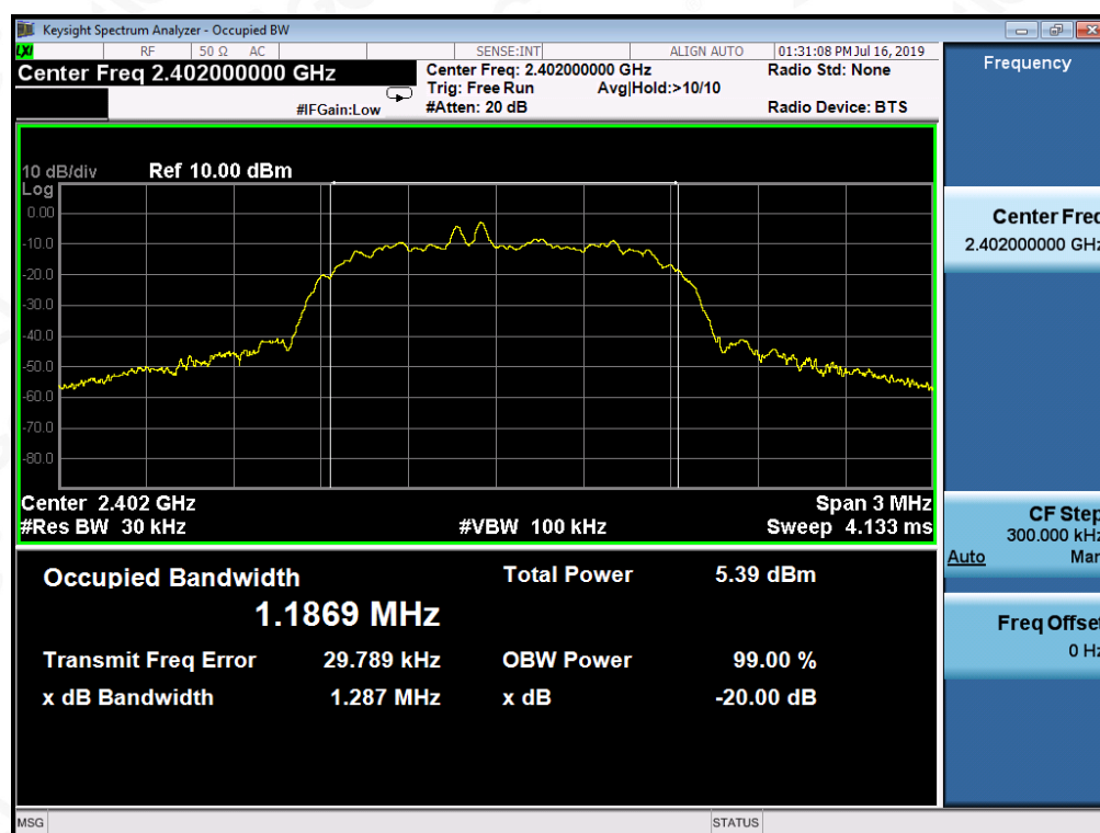
TEST PLOT OF BANDWIDTH FOR LOW CHANNEL
