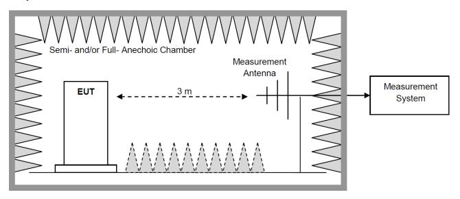
Step 2: Substitution method to verify the maximum ERP/EIRP
