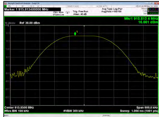
Peak output Power plot on channel 52 (1Mbps)
