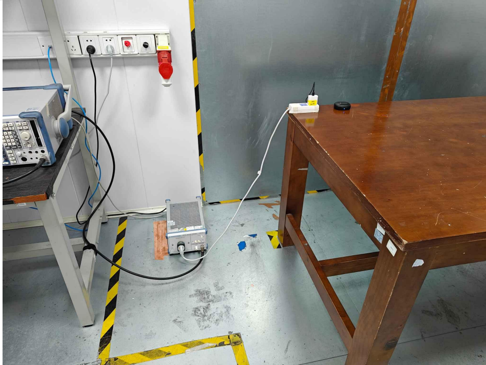
Conducted emissions at AC power line (150kHz-30MHz)
