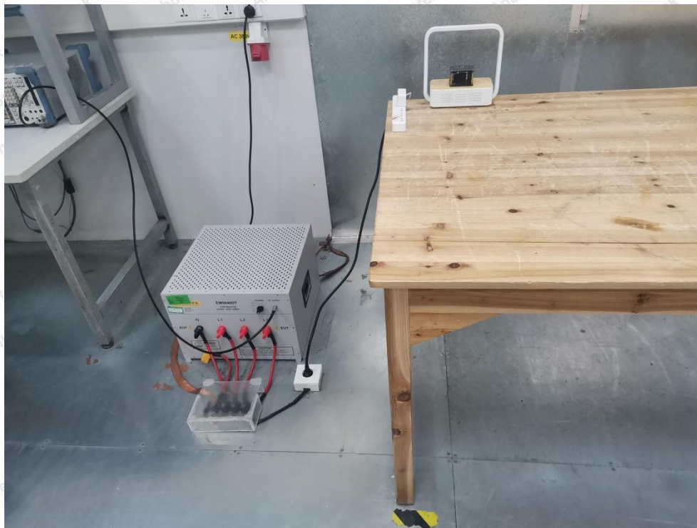
Photo of Conducted Emission Measurement
