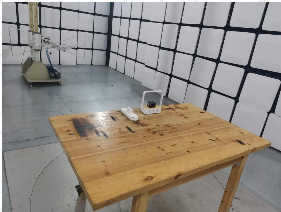
Photo of Radiation Emission Test
