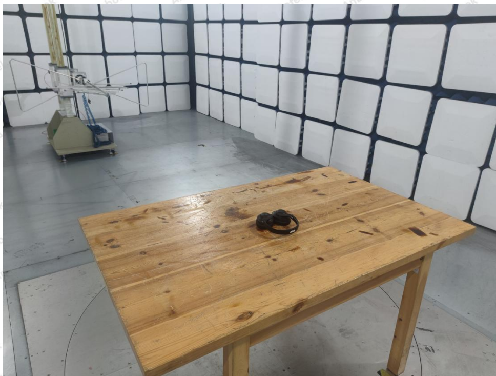
Photo of Radiation Emission Test
