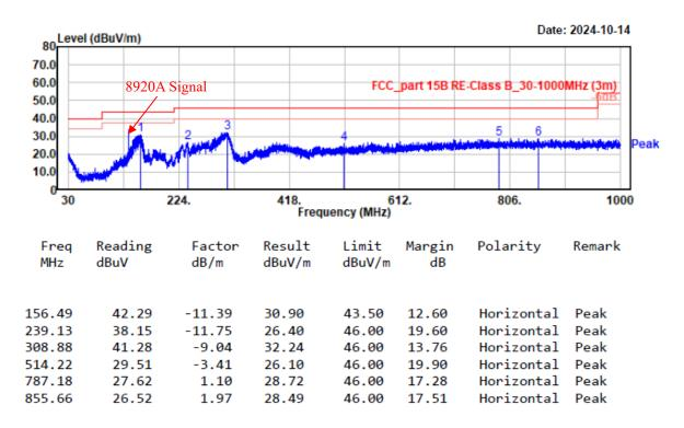
FCC Part 15B Page 21 of 39 Project No.: 2407Y44307E-EM Test Mode: Mode 2(136.0125MHz)
