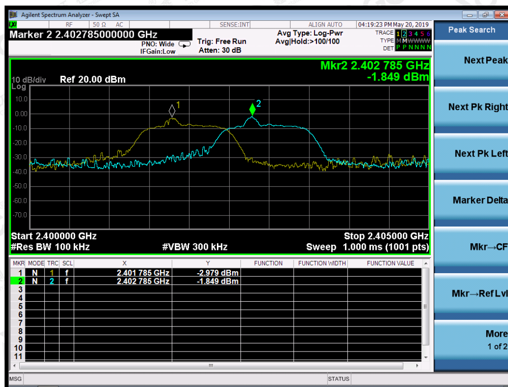
TEST PLOT FOR FREQUENCY SEPARATION
