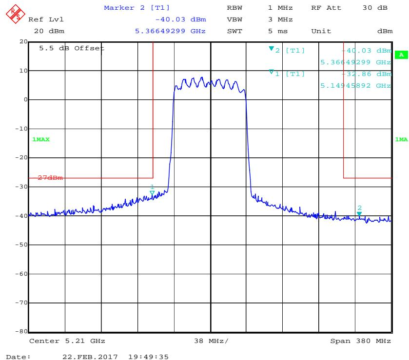
**5725-5850MHz**(the antenna gain was offset in the display, all emissions under limit 3dB, so combined results meet the requirement)
