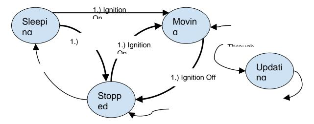
There are 3 main states in the software state machine: Moving, Stopped, Sleeping. There is also an Updating state when the application or settings information on unit are being updated. When in Updating state the device will ignore all normal behavior until unit is updated at which time it is rebooted. The parameters and thresholds applied for state transitions are primarily contained in the Settings File.
