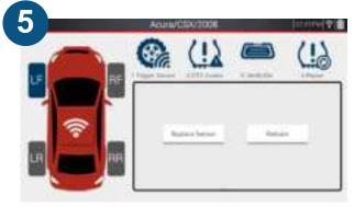
Continuing on to Repair, selecting either Replace or Relearn will take you to that screen at the main TPMS function where you can program a sensor, or perform a relearn
