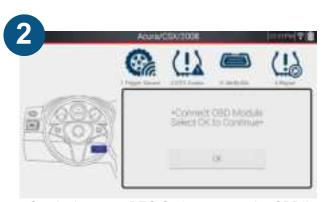
Continuing on to DTC Codes, ensure the OBDII Cable is connected to the tool and vehicle with the ignition in the ON position, Then tap "OK".
