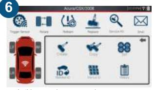
In this example, programming a new sensor is needed. From the program screen, a new sensor can be programmed, and a relearn can be performed if necessary. See section B-4 for programming, and B-2 for relearns.
