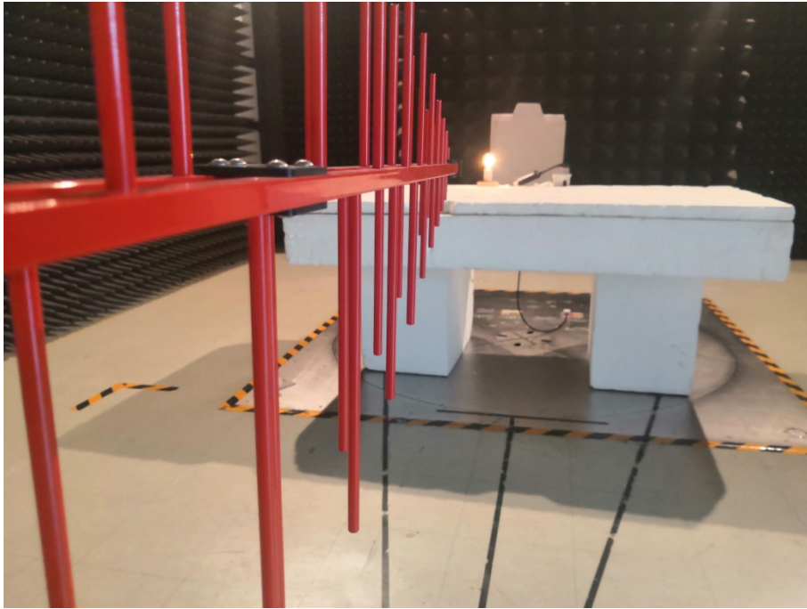
Radiated Emissions -Front View (Below 1GHz)
