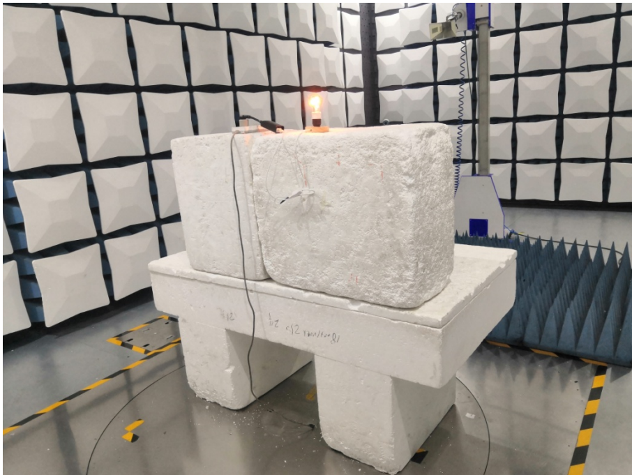
Radiated Emissions - Rear View (Above 1GHz)
