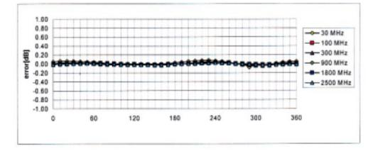
Axial Isotropy Error < ± 0.2 dB
