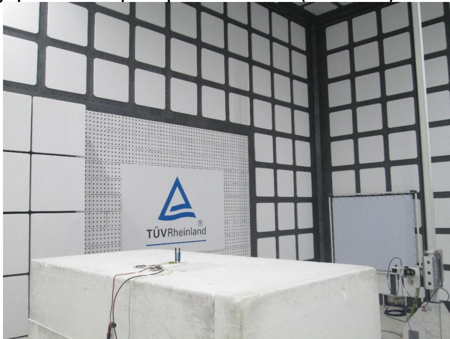
Photograph 6: Test Setup for Spurious Emissions (Back View 4)
