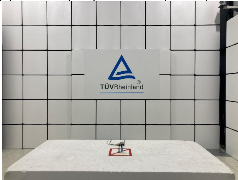
Photograph 10: Test Setup for Spurious Emissions (Front View)
