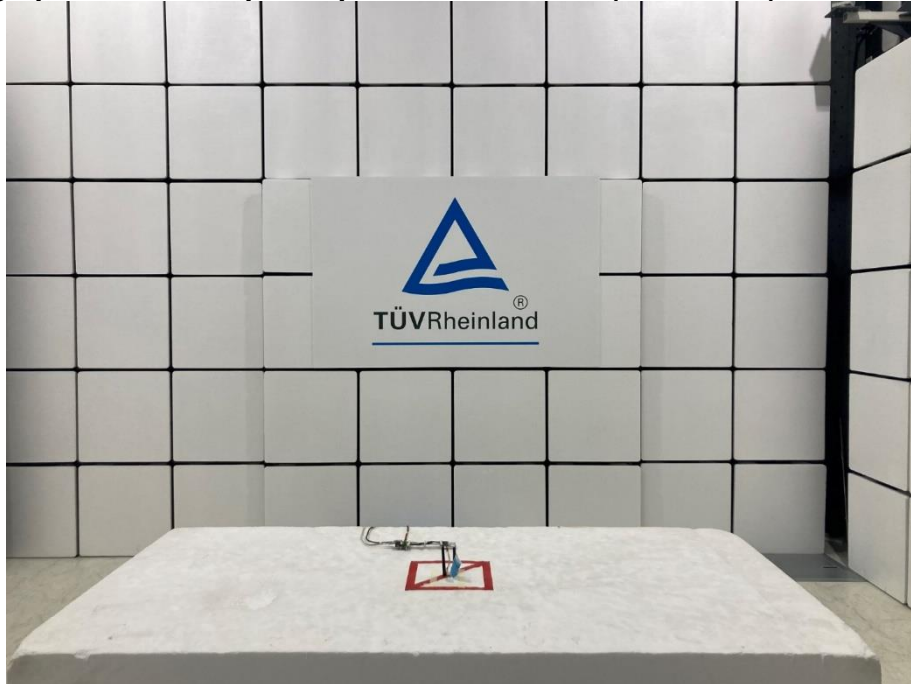
Photograph 7: Test Setup for Spurious Emissions (Front View)
