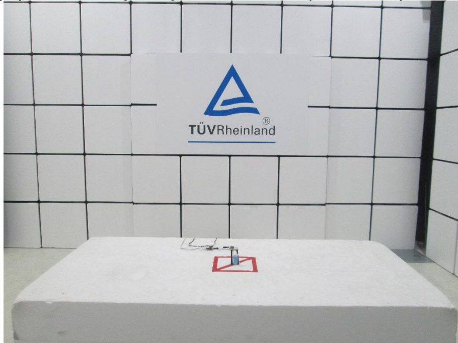
Photograph 1: Test Setup for Spurious Emissions (Front View 1)
