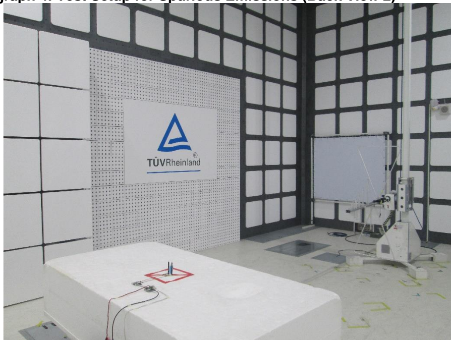
Photograph 4: Test Setup for Spurious Emissions (Back View 2)
