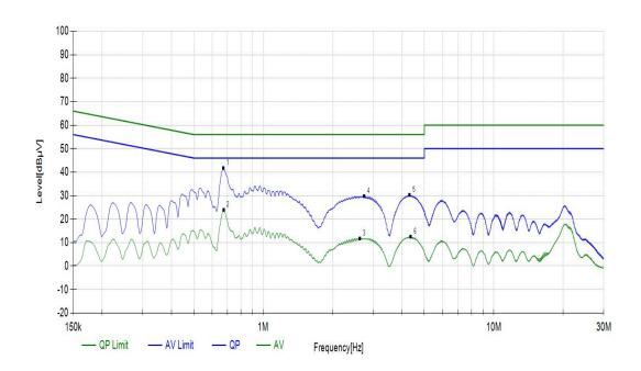
During the test, the Conducted Emission from 150kHz to 30MHz was performed in all modes with all channels, and all antennas. Bluetooth(LE\_1M), Channel 0, Antenna 1 are selected as the worst condition. The test data of the worst-case condition was recorded in this report.
