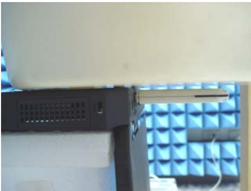
Fig.6 Photograph of the Bottom of the Pc is paralleled and at a distance of 0.0 cm from the base of the phantom.
