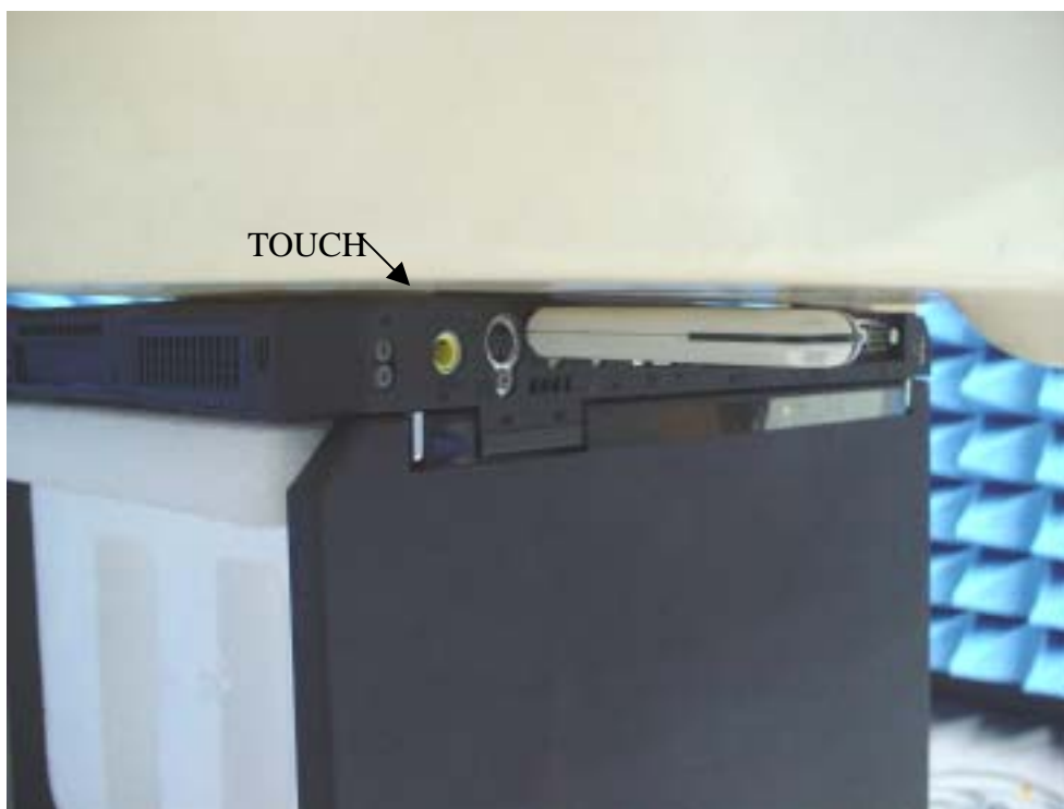
Fig.5 Photograph of the Bottom of the Pc is paralleled and at a distance of 0.0 cm from the base of the phantom.
