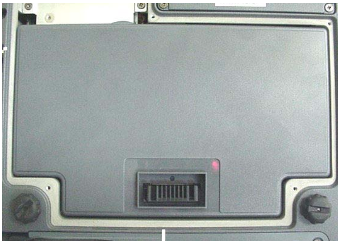
Internal Li-ion Battery 11.1 V, 3600 mAh (Model: T8M-E)
