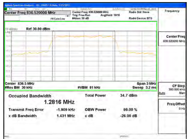
CDMA BC0 1xEV-DO Rev A Middle Channel
