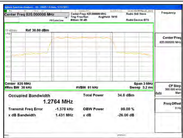
CDMA BC10 1xEV-DO Rev A Middle Channel
