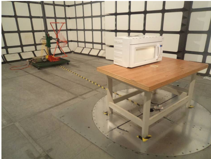
Radiated Emissions - Front View (30 MHz – 1 GHz)
