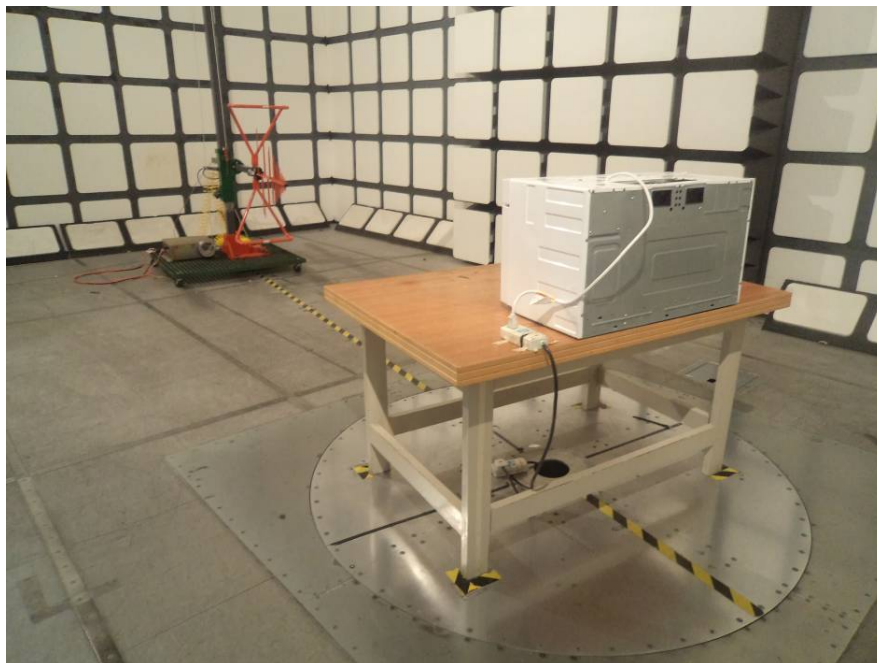
Radiated Emissions - Rear View (30 MHz – 1 GHz)
