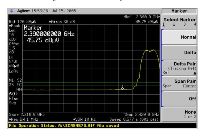
Detector mode: Peak Polarity: Horizontal
