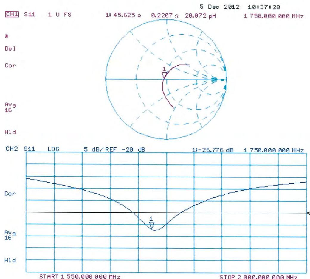
Dipole D1750V2 – SN: 1081 Antenna Parameters measured: 2014-02-21.
