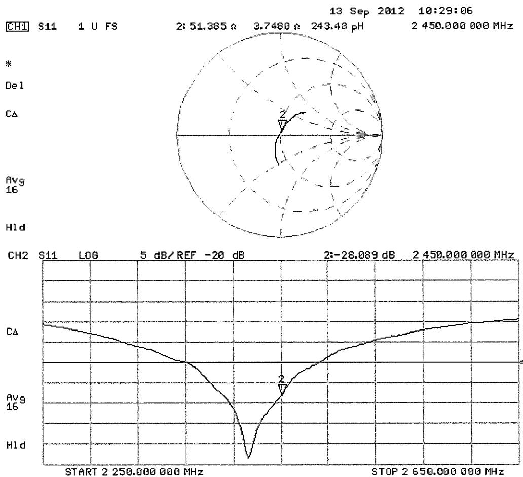
Dipole D2450V2 – SN: 800 Antenna Parameters measured: 2013-10-10.
