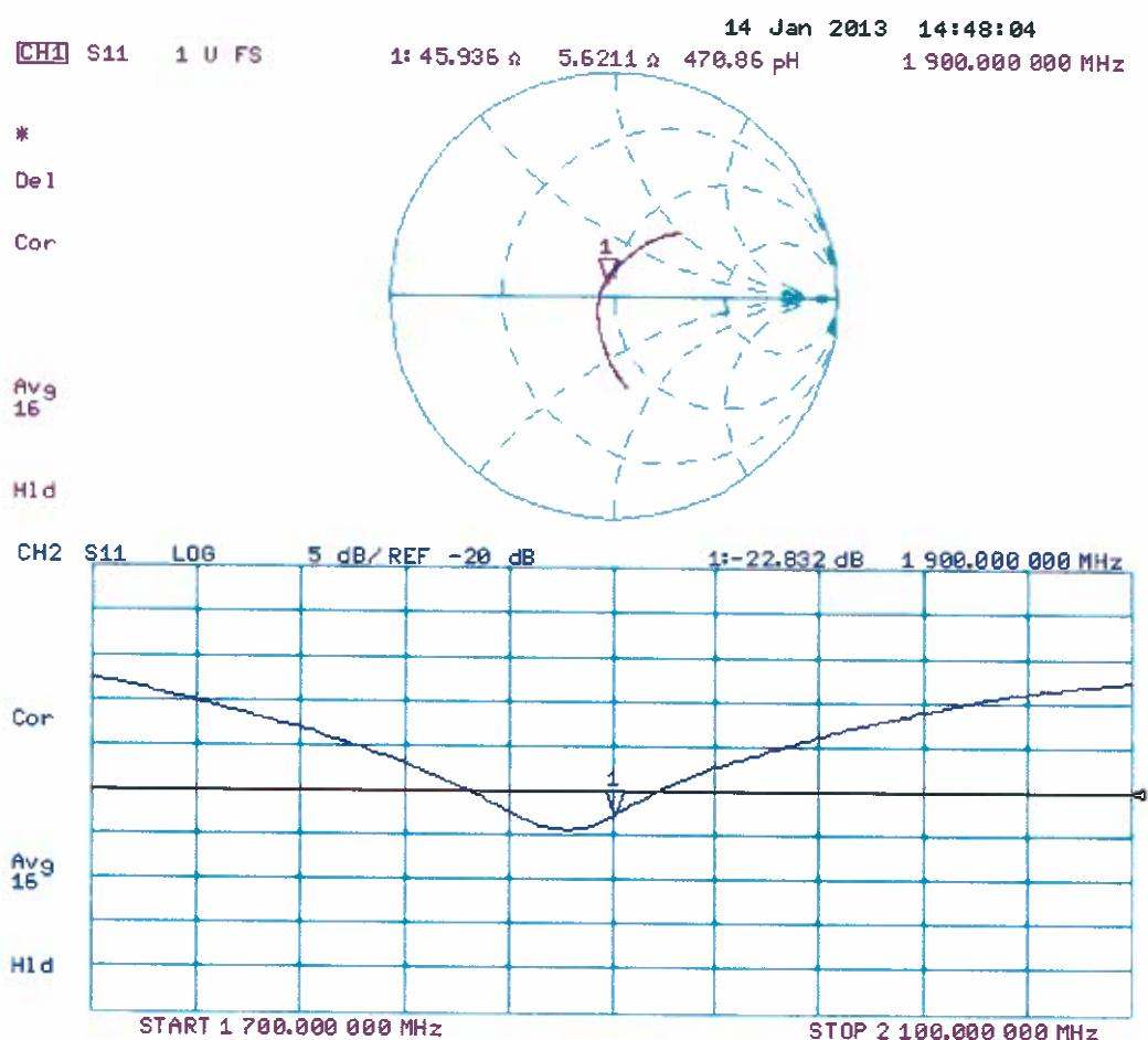
Dipole D1900V2 – SN: 5d099 Antenna Parameters measured: 2014-02-14.
