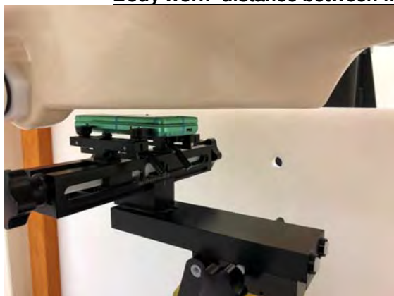
Fig.7 EUT Front side to flat phantom
