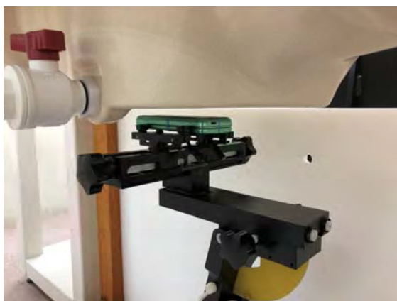
Fig.8 EUT Back side to flat phantom
