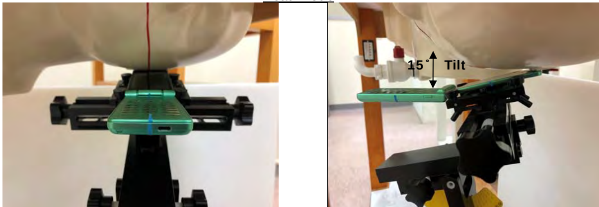
Fig.6 Left Head Section / Ear-Tilt Position(15°)
