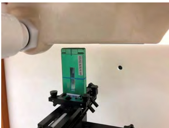
Fig.11 EUT Top side to flat phantom
