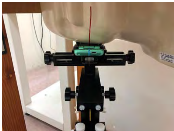
Fig.3 Right Head Section / Cheek-Touch Position
