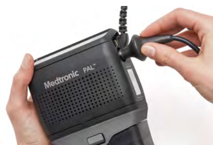
Figure 63: Pull the power cord out
