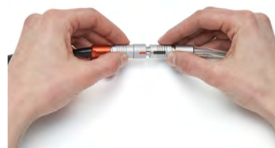
Figure 105: Disconnect the driveline
