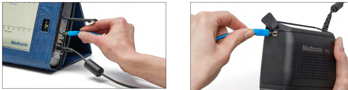
Figure 164: Data cable from monitor to controller
