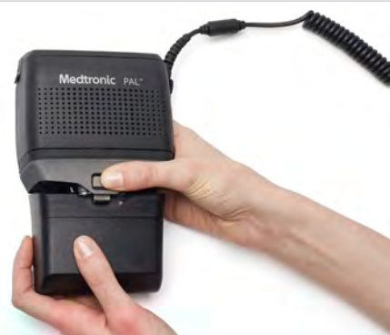
Figure 70: Press the “Battery Release” button
