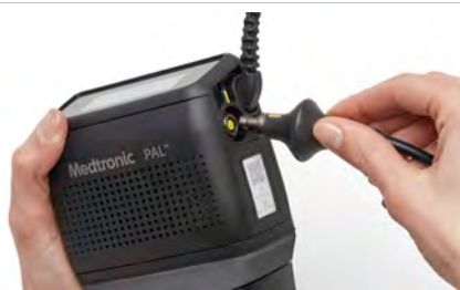
Figure 74: Align the yellow lines
