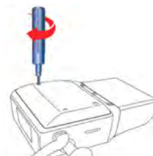
Figure 206: Tighten back cover
