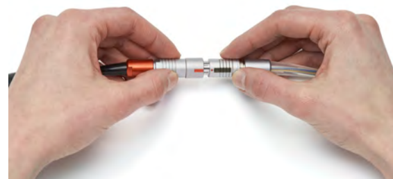
Figure 112: Push the driveline connector into the port
