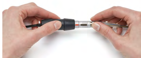
Figure 49: Slide the cover over connectors
