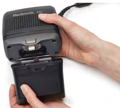
Figure 68: Insert tabs of the battery on the battery connector
