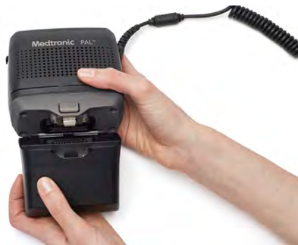
Figure 71: Detach the battery tabs
