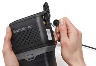
Figure 58: Lift the dust cover
