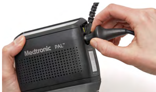
Figure 61: Allow the cable to slide into the controller power connector port
