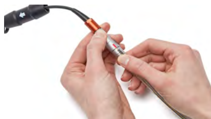
Figure 53: Pinch the grooved area of the controller Coiled Cable connector
