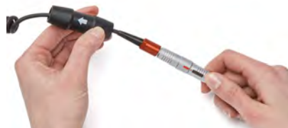
Figure 50: Slide the driveline cover
