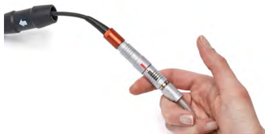
Figure 107: Grasp the pump driveline cable
