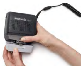
Figure 103: Press button to remove the cap
