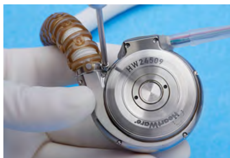
Figure 182: Position the clamp screw to inner side of outflow conduit
