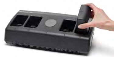
Figure 79: Place battery into charging bay
