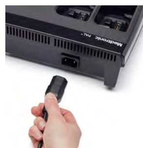
Figure 76: Connect the AC power cord
