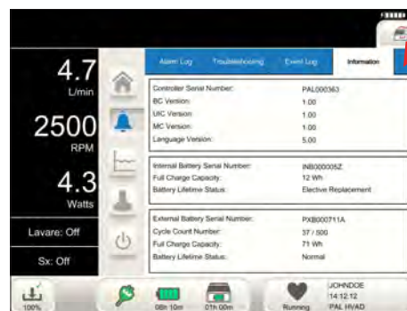
Figure 190: Internal Battery replacement symbol flashing at top right of screen
