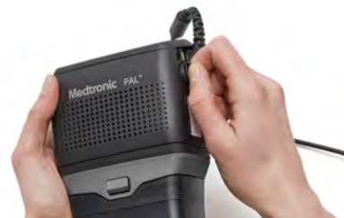
Figure 64: Cover the port with dust cover
