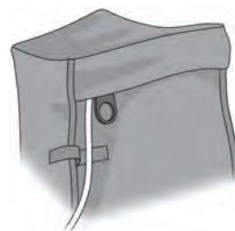
Figure 98: Guide the driveline between the Velcro® strips
