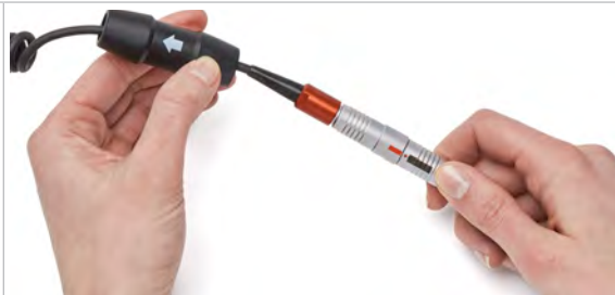
Figure 106: Slide the cover of the pump driveline
