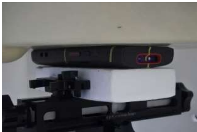
Front Face, Test Separation 0 mm
