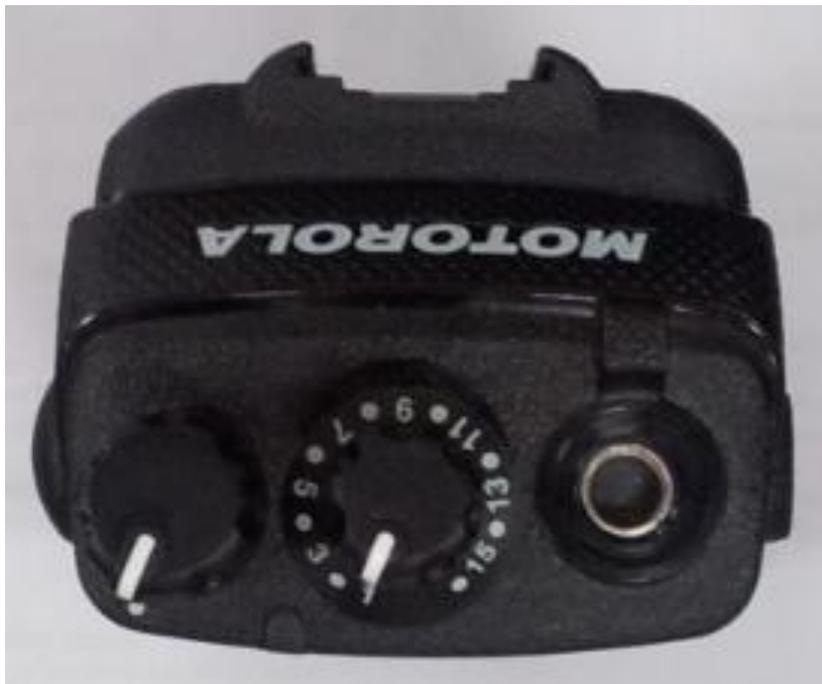
**Top View for Limited Keypad and Plain Model (without Antenna)
