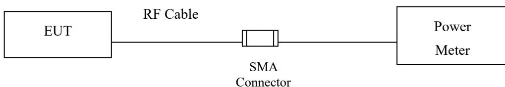
Conduction Power Measurement (for 802.11ac)
