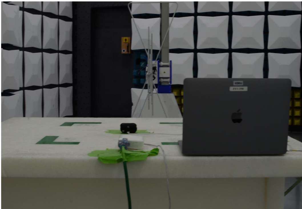
Figure 16: 30MHz-1GHz Test Setup (Rear View)
