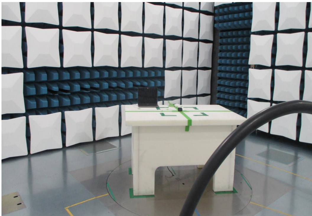
Figure 18: 9kHz-30MHz Test Setup (Front View)
