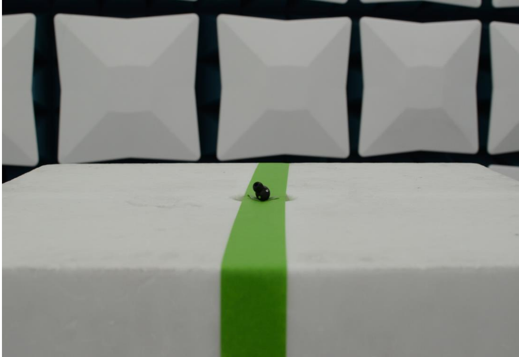
Figure 7: 1-18GHz Test Setup (Front View)
