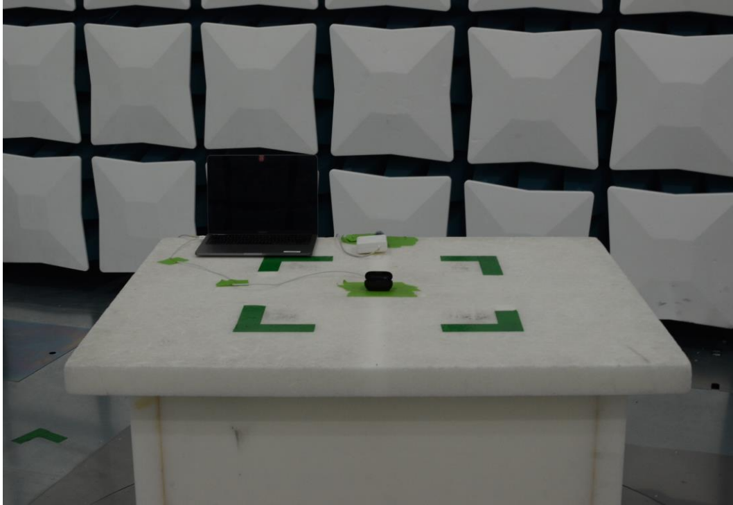
Figure 15: 30MHz-1GHz Test Setup (Front View)
